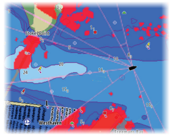
Radar overlay on a chart
