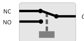
Relay configuration (not energised).
